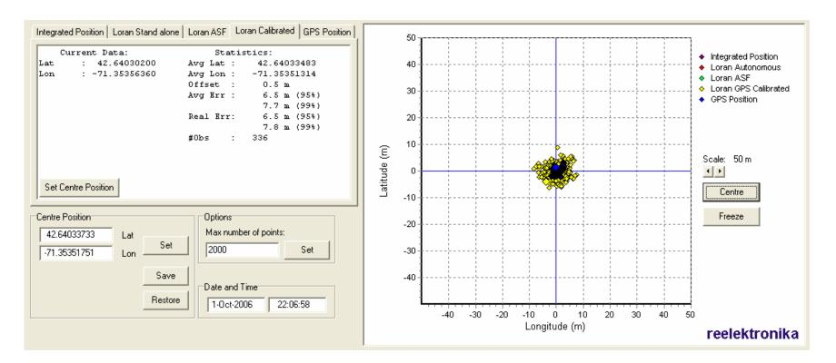
The "calibrated" Loran mode has an error of 6.5m, 95%. The calibrated mode uses GPS data to remove Loran range errors due for each Loran pseudo range. Because it is temporally stable a user can complete operations in the absence of GPS. Alternatives such as mapping or data channel produce similar results.
