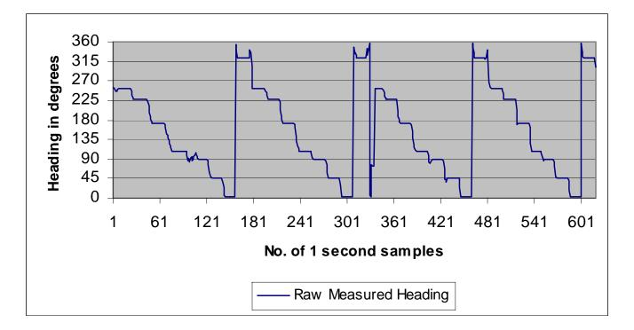
In the Handheld trial the spotter was asked to locate the target and hold it for ten seconds before proceeding to the next target in sequence. The plot above shows all heading measurements for 4 rotations x 8 targets (32 total) in just over ten minutes.
